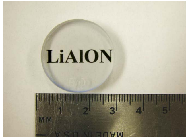
Fig. 8. LiAlON produced by pressureless sintering at 1900^\circ\text{C} for 2 h using a 30 mol% composition initially containing 16 wt.% \text{LiAl}_5\text{O}_8 and then HIPing at 2000^\circ\text{C} for 2 h. The sample is 6.2 mm thick.
